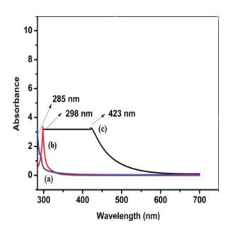
Figure 3 UV-Visible spectra of precursor salt (a), ascorbic acid (b) and Cu NPs (c).
