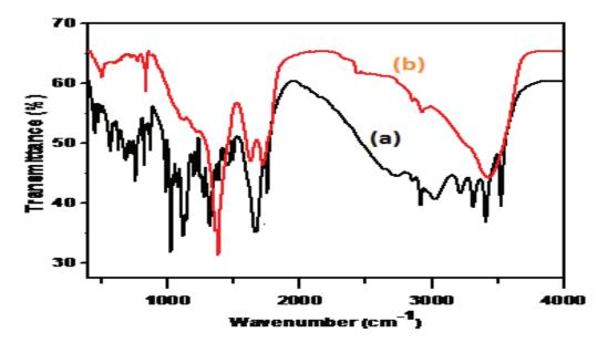
Figure 2 IR spectra of (a) pure L-ascorbic acid and (b) Cu nanoparticles stabilized with L-ascorbic acid
