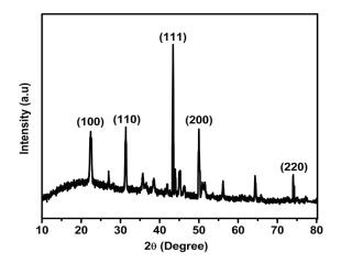
Figure 1 XRD Patterns of the prepared Cu nanoparticles measured with the scanning  $2\theta$  ranges from  $10^{\circ}$  to  $80^{\circ}$ .
