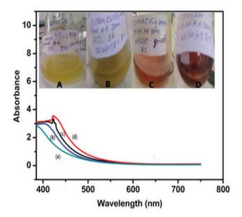
Figure 5 UV-VIS spectra of Cu nanoparticles prepared at (a) 55  $^{\circ}$ C, (b) 65  $^{\circ}$ C, (c) 75  $^{\circ}$ C and (d) 90  $^{\circ}$ C with its corresponding color change
