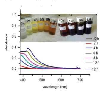
Figure 4 UV-VIS spectra of Cu nanoparticles prepared at different intervals of reaction time with its corresponding color change observed.
