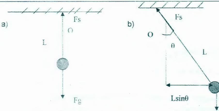
Figure 1: A simple Pendulum at Different States
