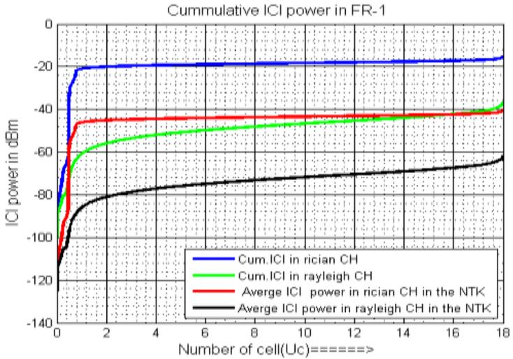
Figure 8. Cumulative and average effect of ICI power under various channel environment for FR-1 network
