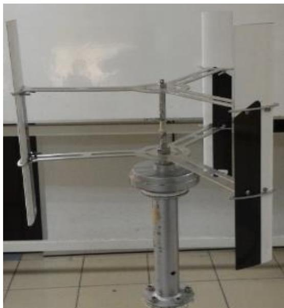
**Figure 2.2:** Lab Scale Model for the VAWT
