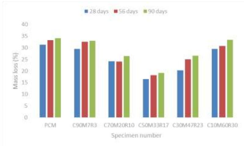
Figure 1: Mass loss of ternary blended GPMs subjected to H<sub>2</sub>SO<sub>4</sub> attack
