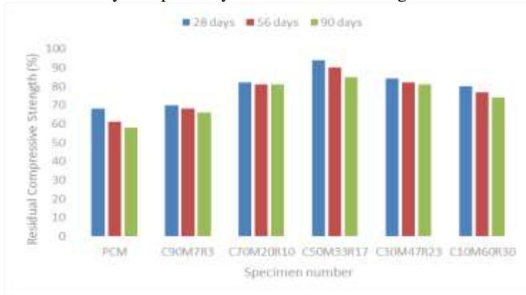
**Figure 2: Strength losses as caused by H<sub>2</sub>SO<sub>4</sub> attack on ternary blended GPMs**
