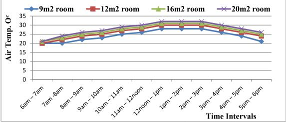
Model 5: Air Temperature of WWR5s for 9m<sup>2</sup>, 12m<sup>2</sup>, 16m<sup>2</sup> & 20m<sup>2</sup>
