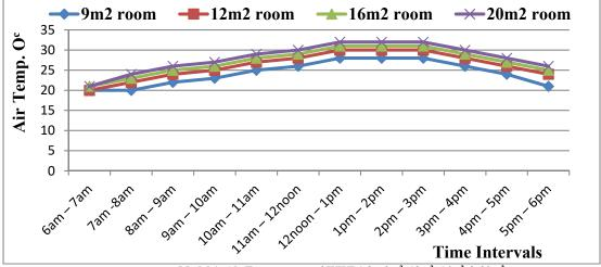
Model 1: Air Temperature of WWR1 for 9m<sup>2</sup>, 12m<sup>2</sup>, 16m<sup>2</sup> & 20m<sup>2</sup>
