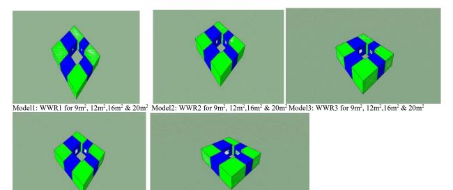
Model4: WWR4 for  $9m^2$ ,  $12m^2$ ,  $16m^2$  &  $20m^2$  Model5: WWR5 for  $9m^2$ ,  $12m^2$ ,  $16m^2$  &  $20m^2$ NOTE: WWR1 = window-size 0.36m<sup>2</sup>, WWR2 = window-size 0.675m<sup>2</sup>, WWR3 = window-size 1.08m<sup>2</sup>, WWR4 = window-size 1.44m<sup>2</sup> & WWR5 = window-size 2.16m<sup>2</sup> respectively. Figure 1: Showing Typology of Simulation Models
