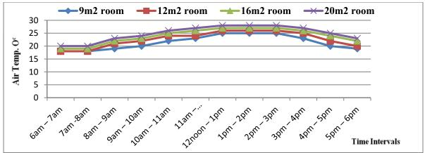
Model 4: Air Temperature of WWR 4 for 9m<sup>2</sup>, 12m<sup>2</sup>, 16m<sup>2</sup> & 20m<sup>2</sup>
