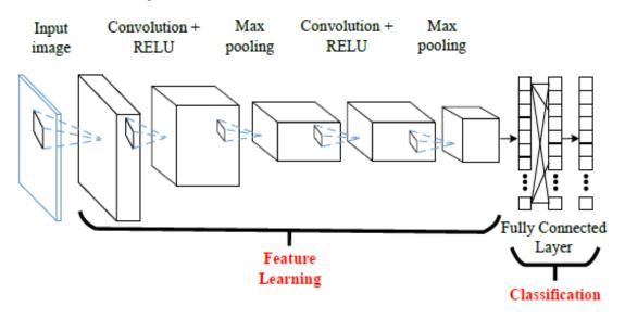
Figure 1: Typical CNN Architecture Source: Kamencay P et. al. (2017).
