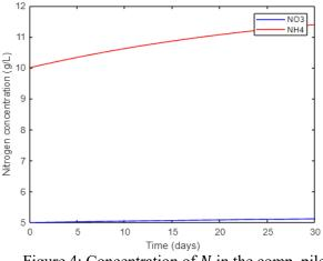
Figure 4: Concentration of N in the comp. pile
