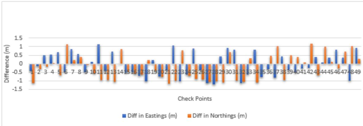
Figure 5: Chart showing computed differences in coordinates of ICP measured on Orthoimage of QuickBird HRSI and ground surveyed GCP
