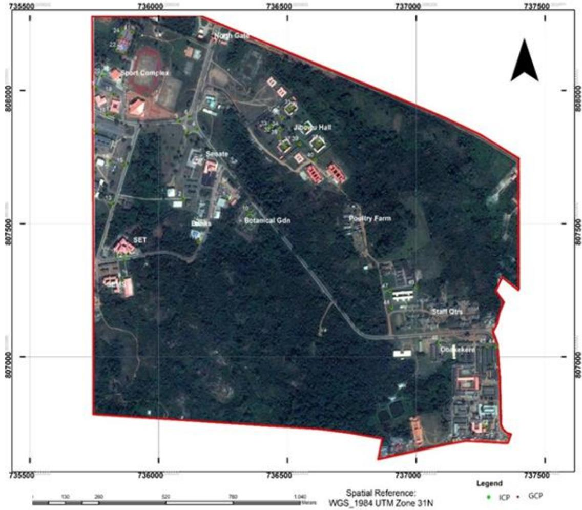
Figure 3: QuickBird-HRSI Orthorectified image map of part of FUTA showing ICP and GCP
