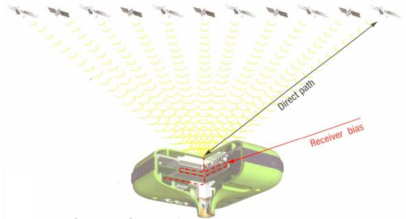
Fig. 3: Receiver biases (Javad GNSS, 2008)
