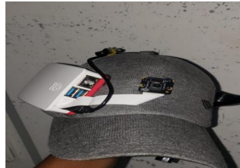
Figure 8: The developed wearable facial recognition system co-integrated on a hat.
