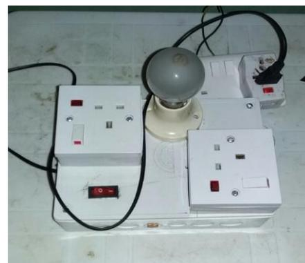
Fig. 7: Pictorial view of Bulb B turned off when there was no Occupant in the room.
