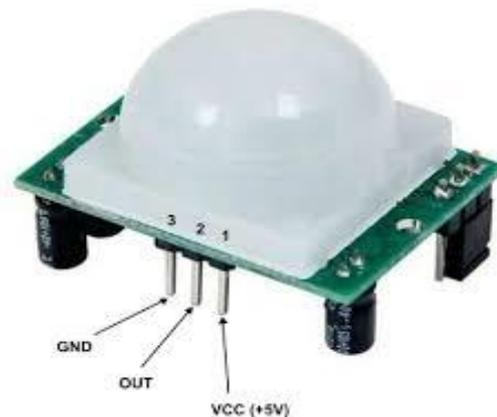
Fig. 2: Pictorial view of the PIR sensor
