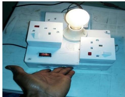
Fig. 6: Pictorial view of Bulb B lit on (though daytime) when there was an Occupant in the room
