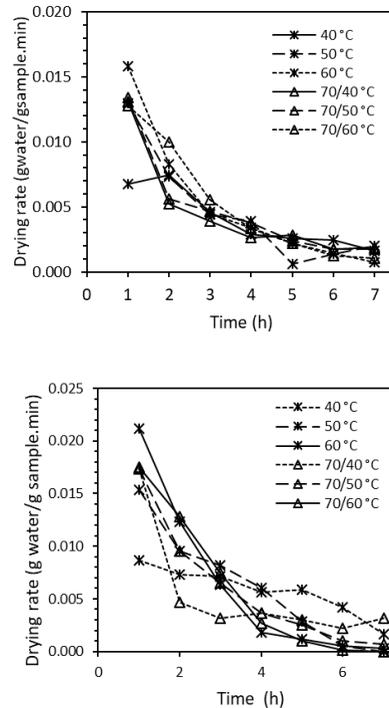
Fig. 2: Drying rate of banana (a) and ginger (b) using single-stage and double-stage drying methods
