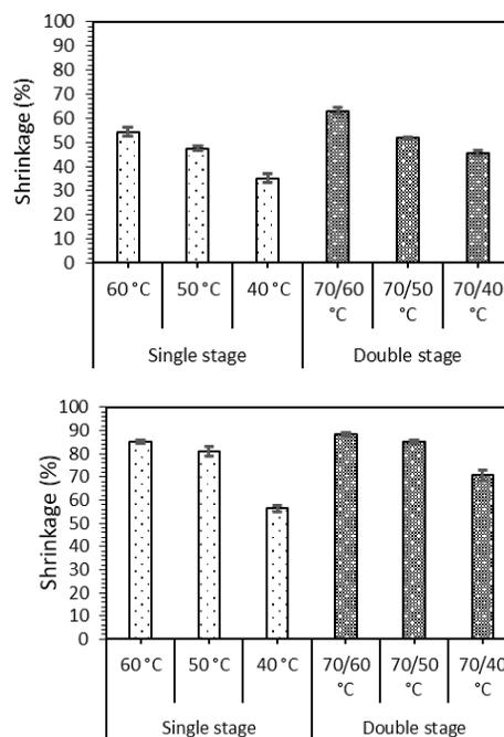
Fig. 3: Extent of shrinkage during single-stage and double-stage drying of (a) banana slices, (b) ginger slices
