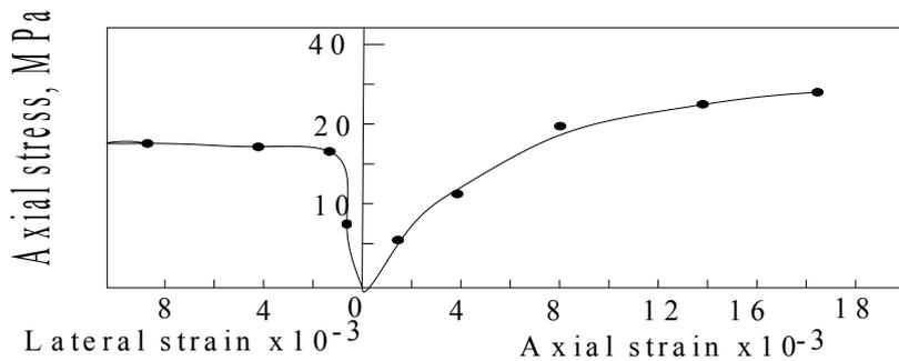
Figure 3.3 Stress strain curves of the fireclay
