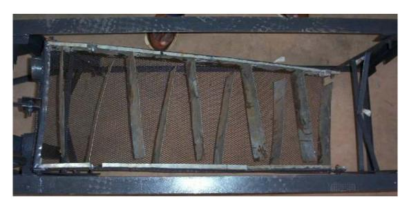
**Figure 8:** Separator tray with baffles inclined at 14 o to the tray axis
