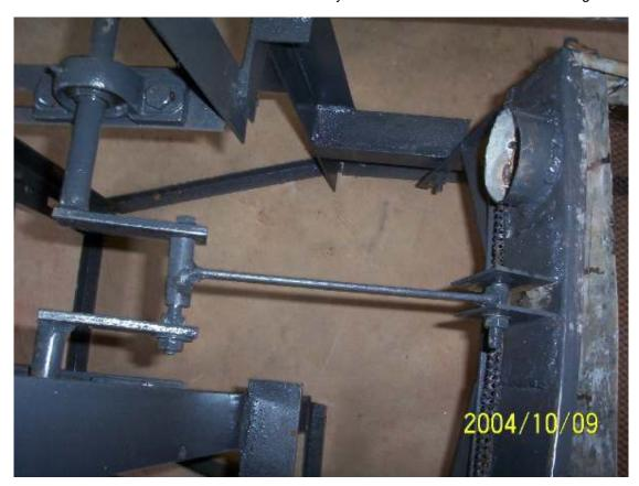
Figure 21: Photograph of the Crank-Rocker Mechanism for agitating the separation chamber
