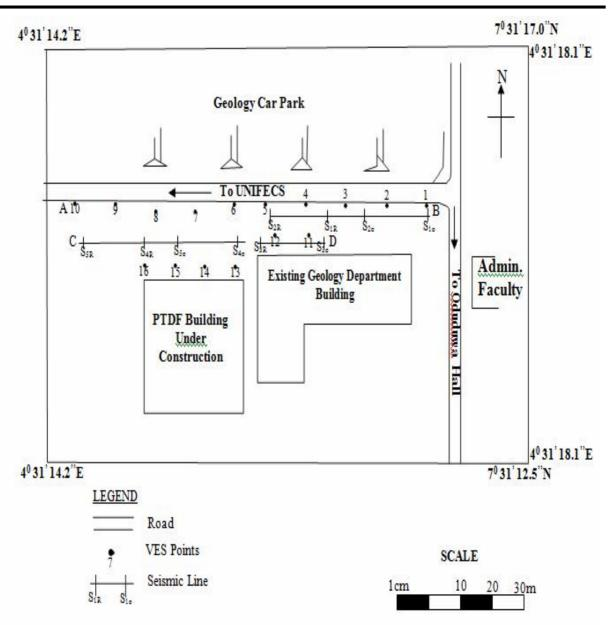
Figure 3: Base map of the study area showing Seismic lines and VES stations
