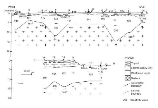
Figure 6: The geoelectric and seismic section of the study area
