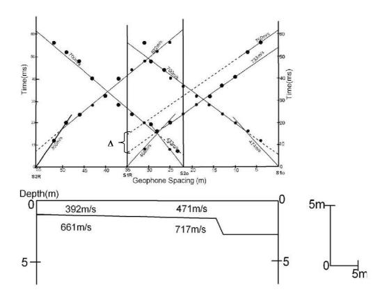
Figure 9: T-X curve of spread 1 and 2
