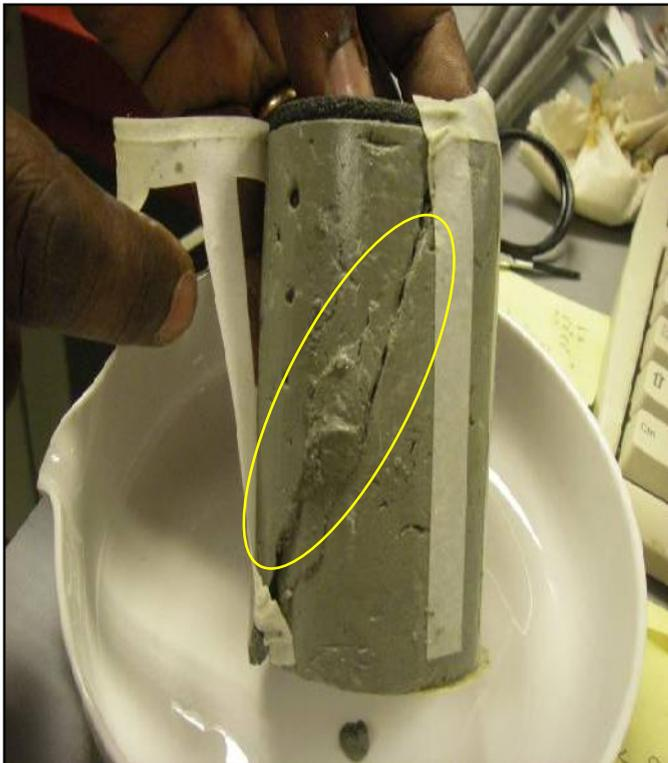
**Figure 8:** Wedging and locking in triaxial failure plane
