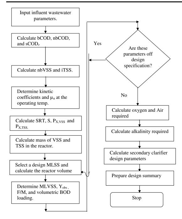
Figure 1: Flow chart for design of completely-mixed activated sludge process for BOD removal and nitrification.
