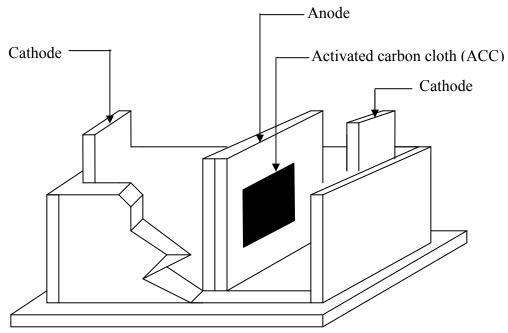
Figure 1 Schematic of electrochemical cell used for electrochemical oxidation.
