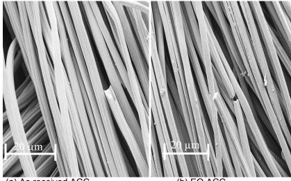
(a) As received ACC (b) EO ACC Figure 6. SEM of ACCs: (a) as -received ACC, (b) EO ACC and (c) ER ACC.
