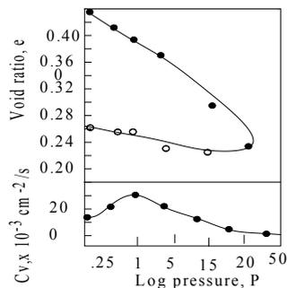
Figure 3.4 Void ratio-, Cv-Log P curves of the indurated fireclay
