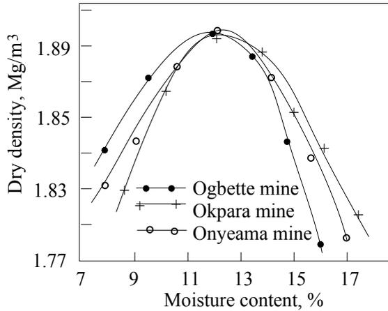
Figure 3.2 Compaction curves of the fireclays
