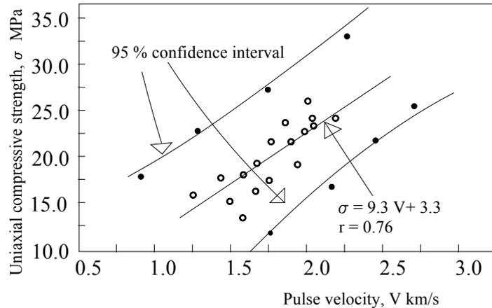
Figure 3.5 Dependence of the unconfined compressive strength,  $\sigma$  on the ultrasonic pulse velocity,  $V$  of the fireclay
