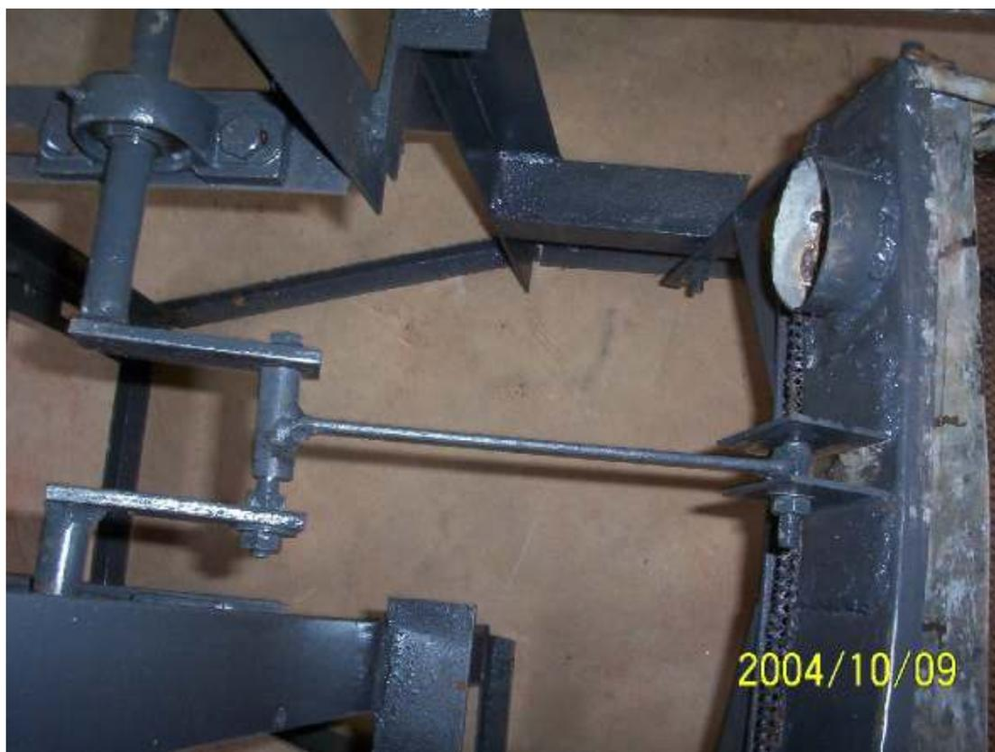
**Figure 21:** Photograph of the Crank-Rocker Mechanism for agitating the separation chamber
