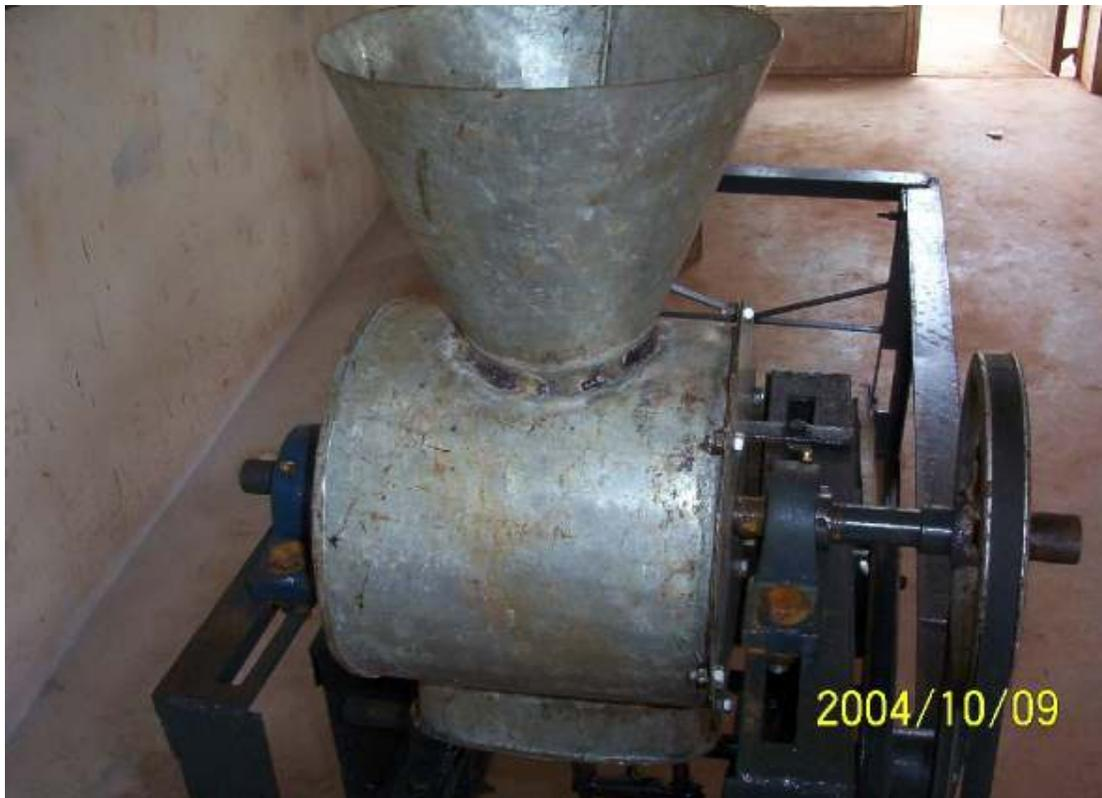
Figure 20: Photograph of the hopper and depulping chamber
