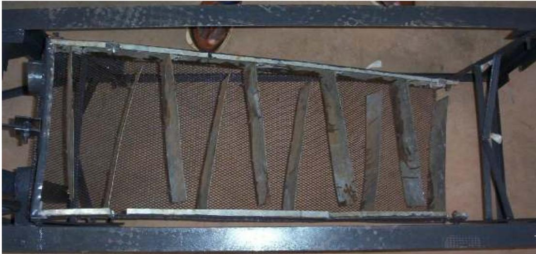
**Figure 8:** Separator tray with baffles inclined at  $14^\circ$  to the tray axis
