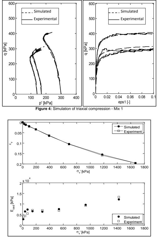
Figure 5: Simulation of oedometer strain and modulus - Mix 1
