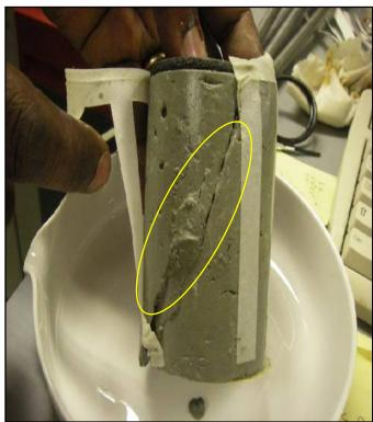
Figure 8: Wedging and locking in triaxial failure plane
