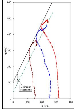
Figure 9: Typical triaxial results showing c-softening
