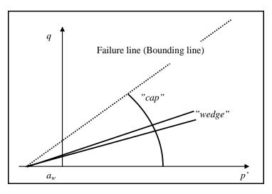
Figure 1: Model principle, visualized in p'-q space
