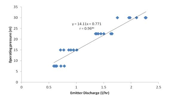
Fig 3. Relationship between operating pressure and emitter discharge for plugged end laterals.
