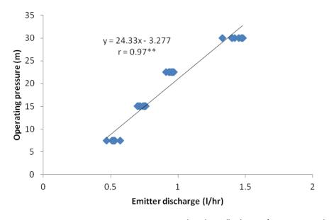
Fig. 1. Relationship between operating pressure and emitter discharge for an opened end lateral.
