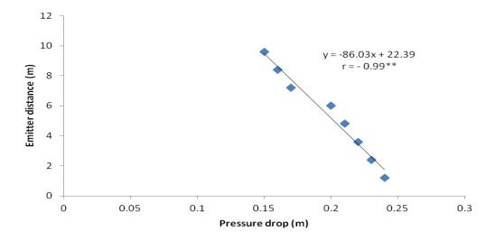
Fig. 4. Relationship between emitter distance (spacing) and pressure drop for plugged end laterals.
