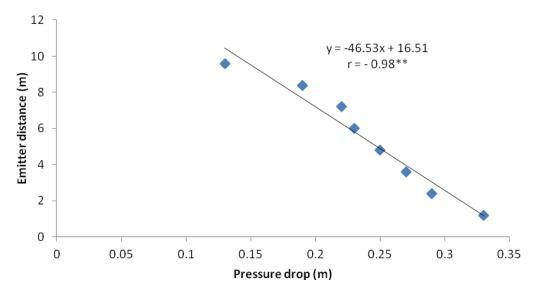
Fig. 2. Relationship between emitter distance (spacing) and pressure drop for an opened end laterals.
