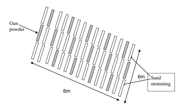
Figure 2: View showing distribution of Gun Powder in the Basal part of the bench
