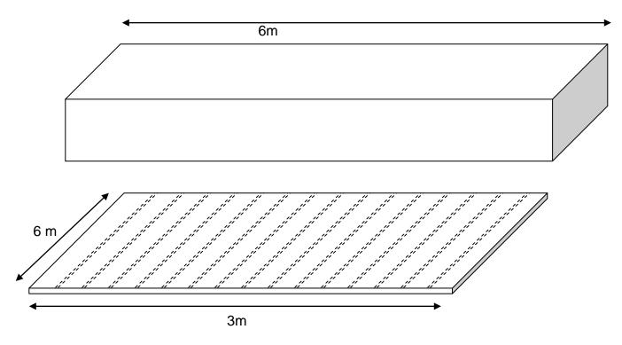
Figure 5: View showing Pattern 3 of Dynacord distribution in the Basal of the bench
