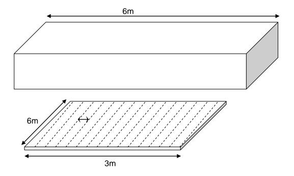
Figure 3: View showing pattern 1 of Dynacord distribution in the Basal of the Bench.
