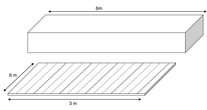
Figure 6: View showing Pattern 4 of Dynacord distribution in the Basal of the bench.
