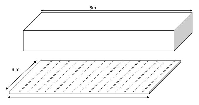
Figure 4: View showing pattern 2 of Dynacord distribution in the Basal of the Bench
