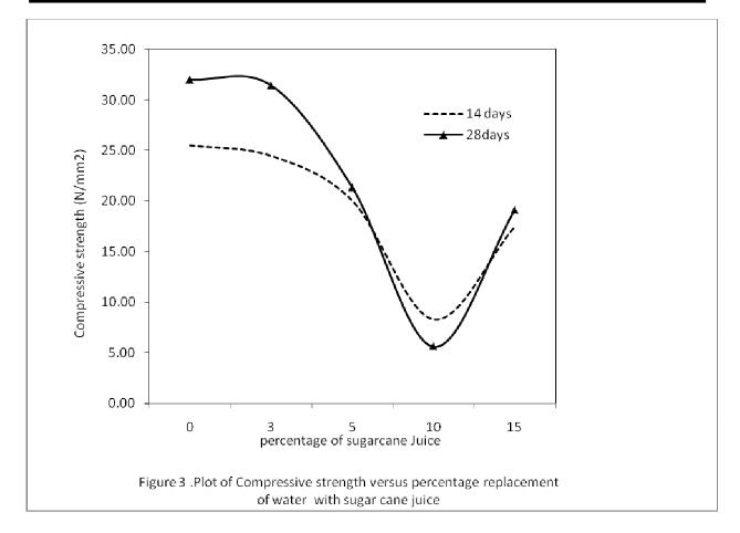
(Neville et al, 2006) observed that sugar when used as a retarder severely reduces early strength of concrete for all ages, thereafter the strength increases at all ages. The early decrease in strength is due to quick-setting. As the quantity of SCJ increases, retardation sets in leading to increase in strength. The result of the current study is in agreement with the above fact.
