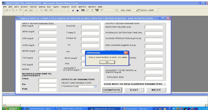
Figure 4: Graphic user interface for error control (no entry).
