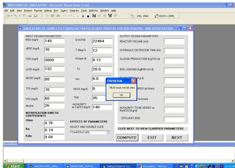
Figure 6: Graphic user interface for error control (zero entry for certain parameters).
