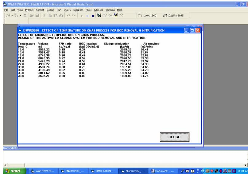
Figure 8: Effect of temperature on BOD removal and Nitrification.
