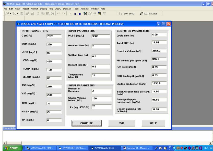
Figure 9: Graphic user interface showing results for sequencing batch reactor.
