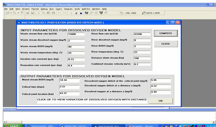
Figure 10: Graphic user interface showing results for dissolved oxygen model.
