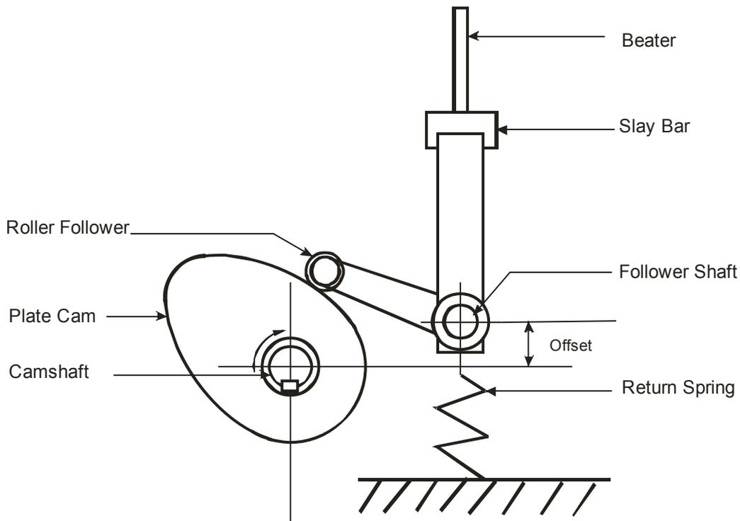
**Fig. 1:** Schematic diagram of the Model Mechanism.
