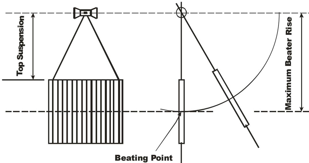
Fig. 2: Schematic View of the Primitive Beater.
