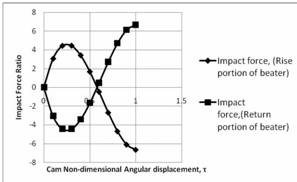
Fig. 4: Plot of the Beater system Impact Force against Cam angular Displacement
