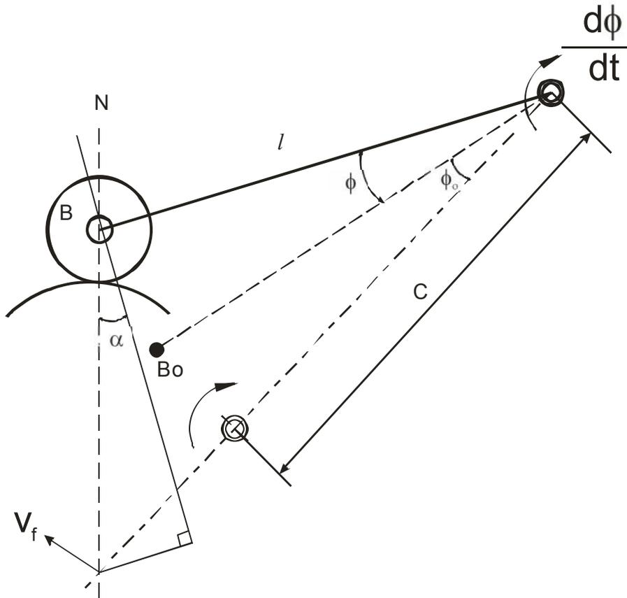
Fig. 3: Geometric Layout for Pressure Angle.
