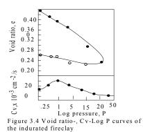
The compression index represented by the slope of the void ratio-log P curve, and designated  $C_c$  is given as:
