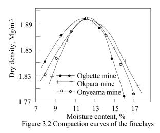
Residual lateritic clays over granite in the Auchi – Afowa area of Edo State, Nigeria have earlier been shown to have negative liquidity index (Ilugbekha, 1989). The dry density-moisture content curve of Fig. 3.2 is typical of clays and shows a maximum dry density of 1.83 Mg/m<sup>3</sup> at optimum moisture content of 12.3%.
