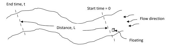
Figure 1: Float-method set up for measuring the river flow
