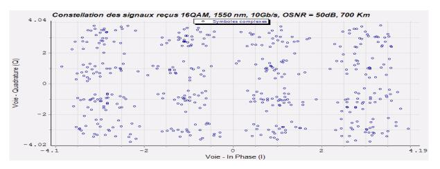
Figure 4: 16QAM received constellation, 1550nm, 10Gbps, OSNR = 50dB
