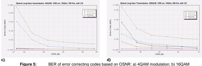
BER of error correcting codes based on OSNR: a) 4QAM modulation; b) 16QAM modulation; c) 64QAM modulation; d) 256QAM modulation.
