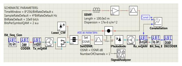
Figure 2: Scheme of the simulation in VPITransmissionMaker 8.7
