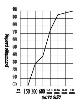
Figure 1. Grading curve for the river sand
