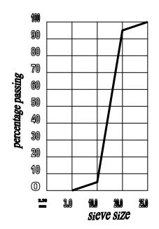
Figure 2. Grading curve for the crushed granite
