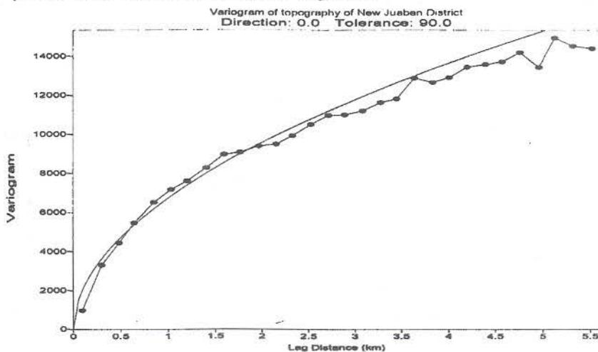
Fig. 2. Experimental Variogram fitted with the power model
