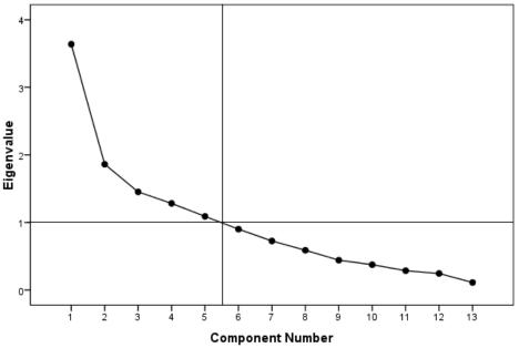
Fig 2: Scree plot showing the eigenvalues sorted from large to small as a function of the principal component number
