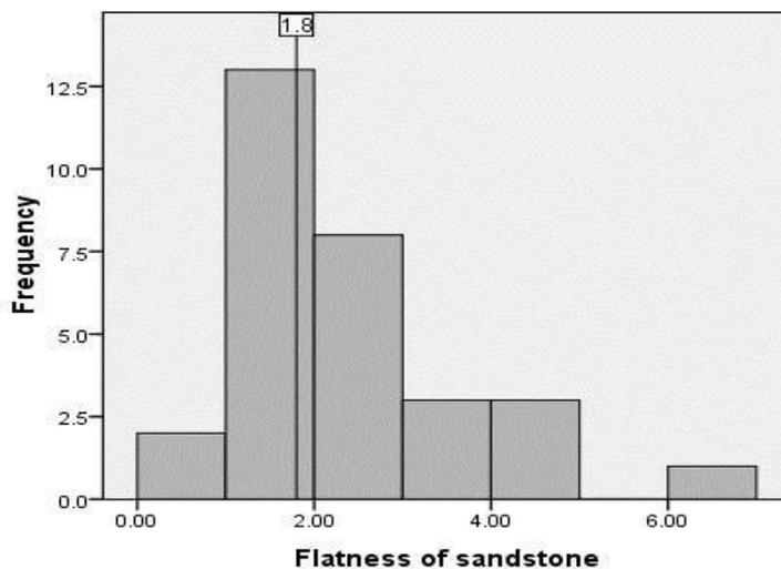
**Figure 6: A histogram showing the flatness of Elmina sandstone**
