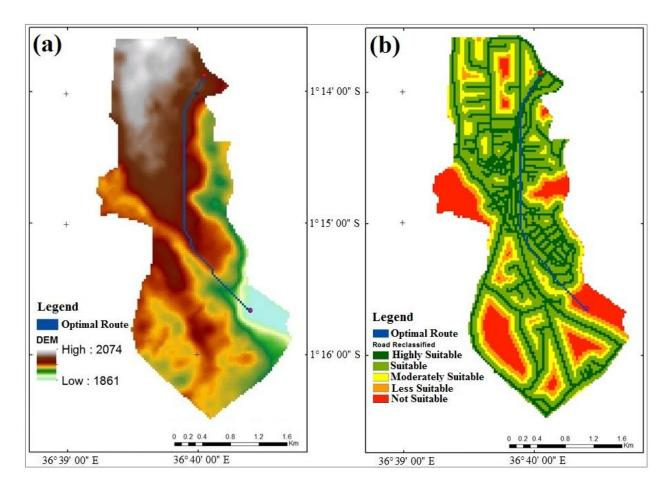
Figure 5: Effects of DEM (a) and Roads (b) on Sewer-line Route
