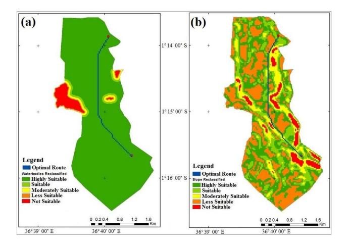
Figure 4: Effects of Water Bodies (a), Slope (b) on Sewer-line Route
