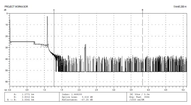
Figure 3: OTDR Event tracing of scenario three
