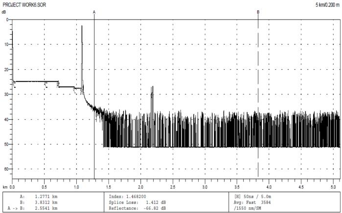
Figure 1: OTDR Event tracing of scenario one
