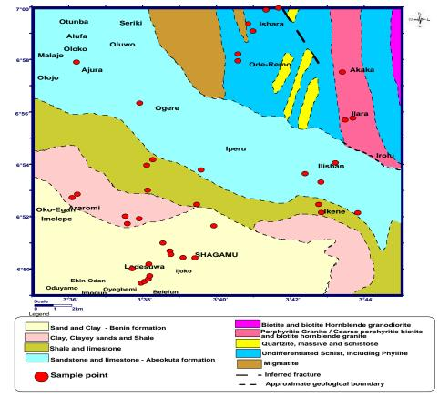
Fig 1: Geological Map of the study area showing sampling points (Modified from Carter, 1964)
