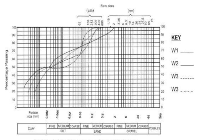
Fig: 3. The Grain size distribution curves for analyzed soil samples
