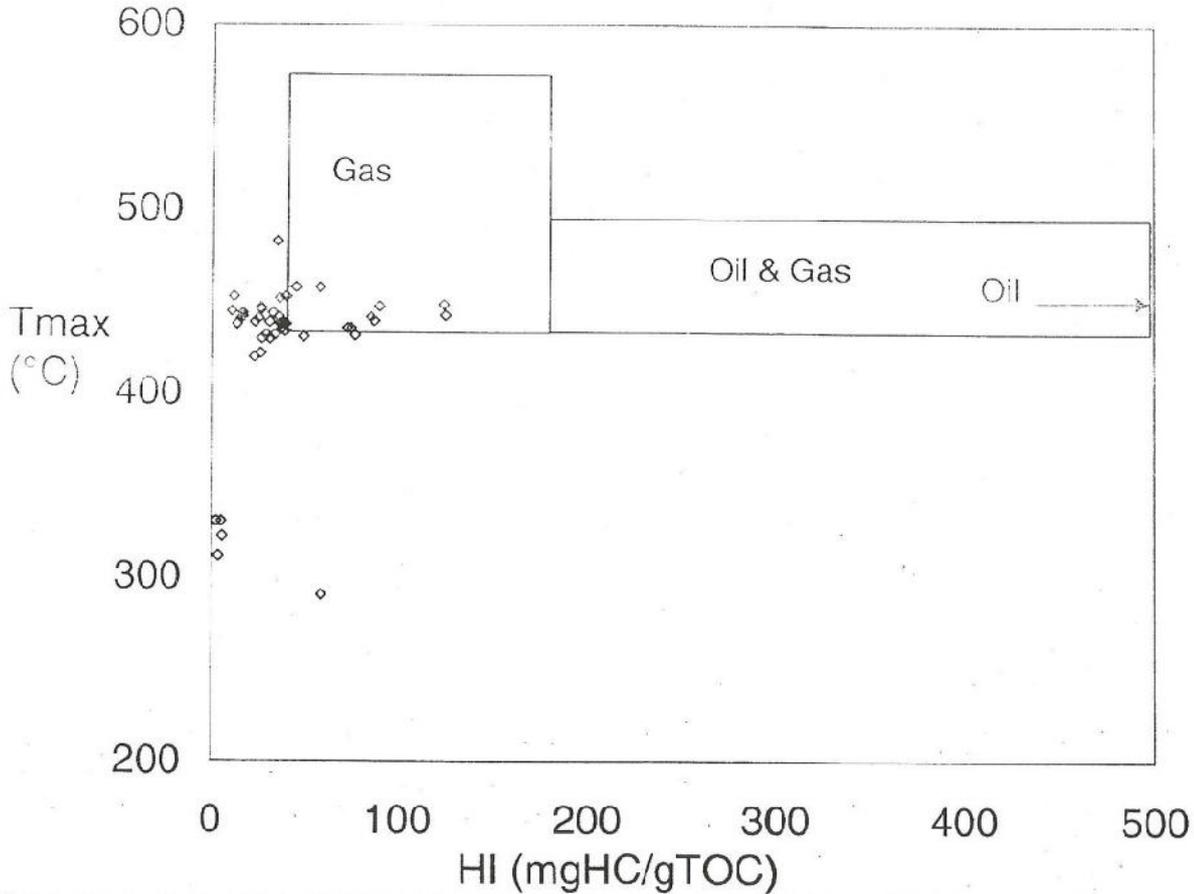
**Figure 7:** HI-Tmax plots of samples from Bornu Basin (diagram constructed based on values given by Peters (1986) depicting entirely gas generative potential and organic matter in most of the samples as inert.
