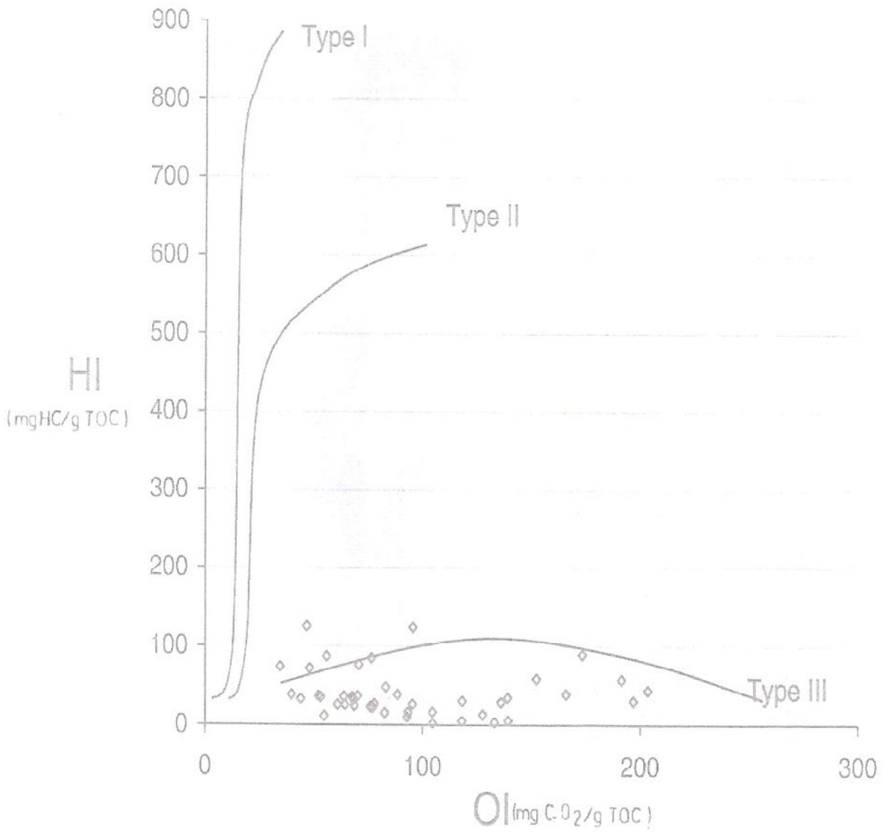
**Figure 6:** HI vs OI plot of the modified Van Krevelen diagram of samples from the Bornu Basin.
