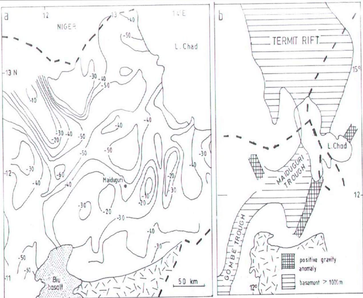
**Figure 3:** a, Bouguer gravity anomaly map of the Bornu Basin (Contours at 10mGal intervals) (Simplified from Cratchley *et al.*, 1984 and Avbovbo *et al.*, 1986). b, Generalized structural interpretation of the Bornu Basin and adjacent areas on basis of geophysical data (Simplified from Cratchley *et al.*, 1984), (After Zaborski *et al.*, 1997).
