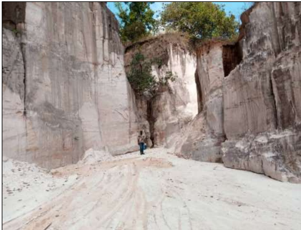
Fig 4.13b: Ajali Formation sandstone unit exposed at Ezi Edda sand mine pit. It is fine – medium-grained, well-sorted, and poorly cemented.
