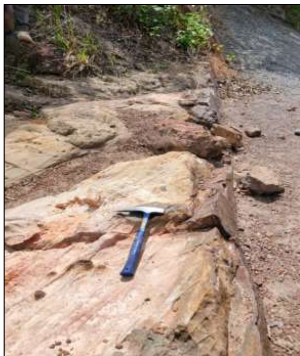
Fig 4.14: Strike-slip fault at Nguzu hill, this could provide a migration pathway and seal.
