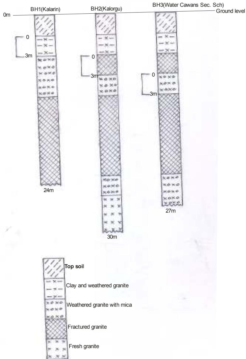
Fig. 3 Lithologic sections of some boreholes in the study area
