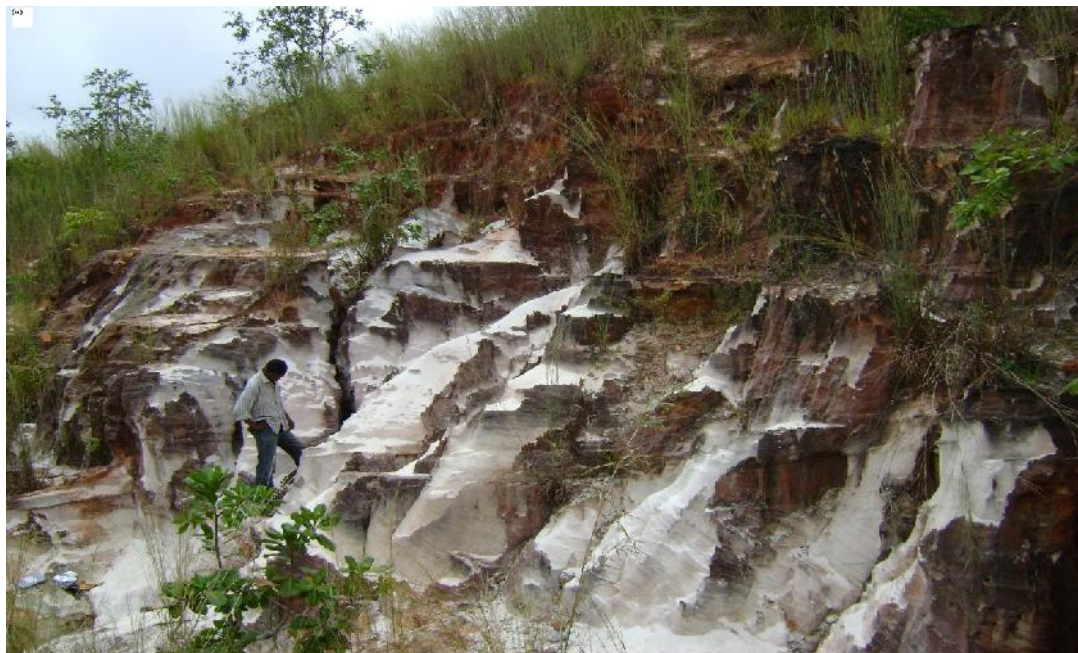
Fig. 2: Field photograph of the sandstone outcrop at location 5 (Fugar). Note the prominent cross stratification of the beds and friable nature of the rock.
