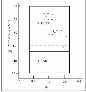
Fig. 3. Environmental determination using bivariate plot of pebble roundness (%) vs elongation ratio (I/L) (After Sames)
