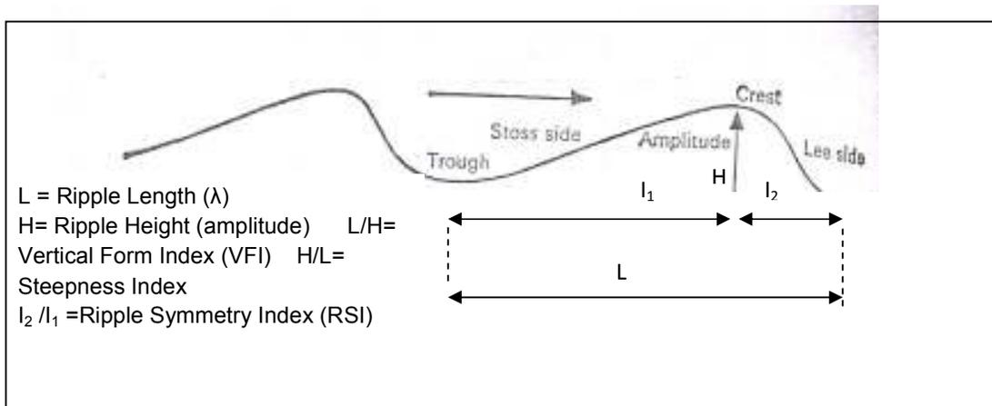
Fig.3: Sketch diagram showing ripple parameters measured in the field.
