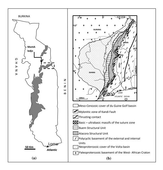
**Figure 1** : Geographic location and geological setting of the Aledjo Mountains: a- zone of the principal reliefs (altitude > 600m) of the framework of the Dahomeyide Belt in Togo ("Mount Togo"); b- frontal units of the Dahomeyide orogen thrust on the Volta Basin which rests unconformably on the south-eastern margin of the West-African Craton.
