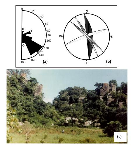
**Fig 3:** Some aspects of fracturing in Aledjo quartzites. (a) rose diagram of the distribution of fracture planes (O = oblique, L = longitudinal and T = transverse); (b) cyclographic traces of median planes of the different fracture families; (c) example of hectometric strike-slip faults responsible for photofacies of the Aledjo Mountains.
