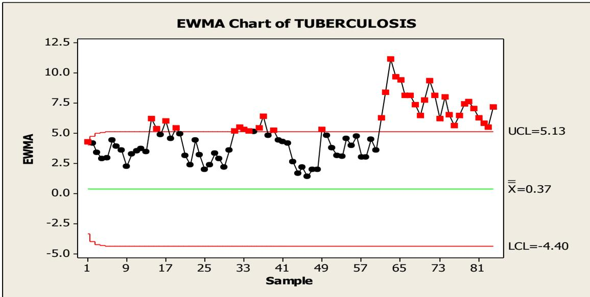
**Figure 8:** EWMA control chart for  $w = 0.15$
