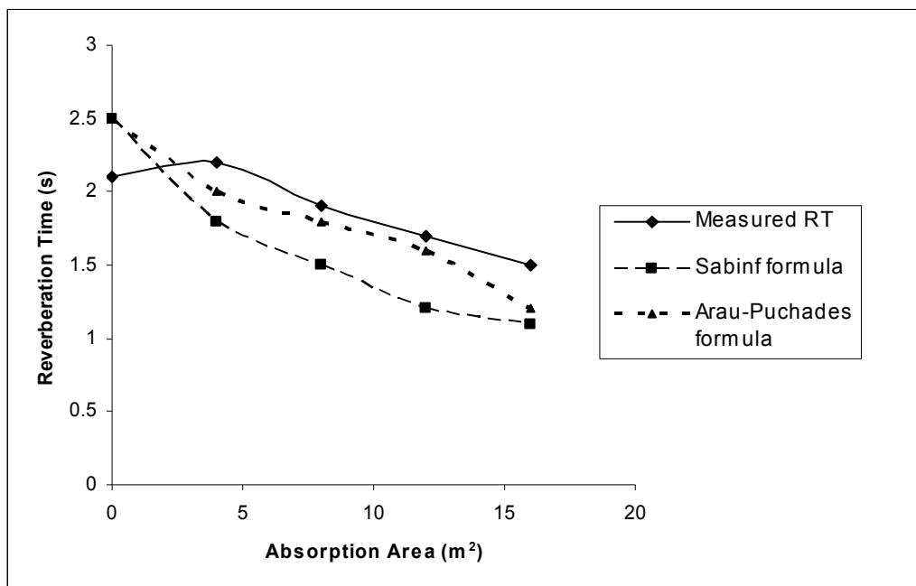
Fig. 1: The Variation of Reverberation Time with Absorption Area of Specimen at 500Hz. Measured reverberation time is given by the full curve, calculated
