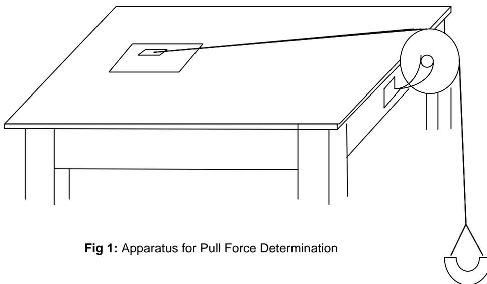
Fig 1: Apparatus for Pull Force Determination
