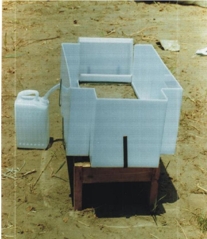
Plate 1: Complete Set of Soil Tray with Splash Collectors Attached
