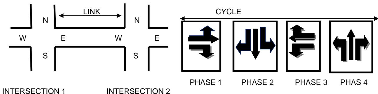
**Figure 1:** Graphical representations showing Link, Cycle and Phase in a typical traffic lights control system
